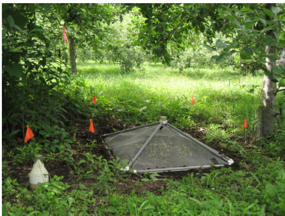
Figure 1. Depiction of the polyvinyl chloride (PVC) enclosure (left) and pyramidal emergence cage (1 m × 1 m at the base) (center) used for the evaluation of entomopathogenic nematodes in the second study.
