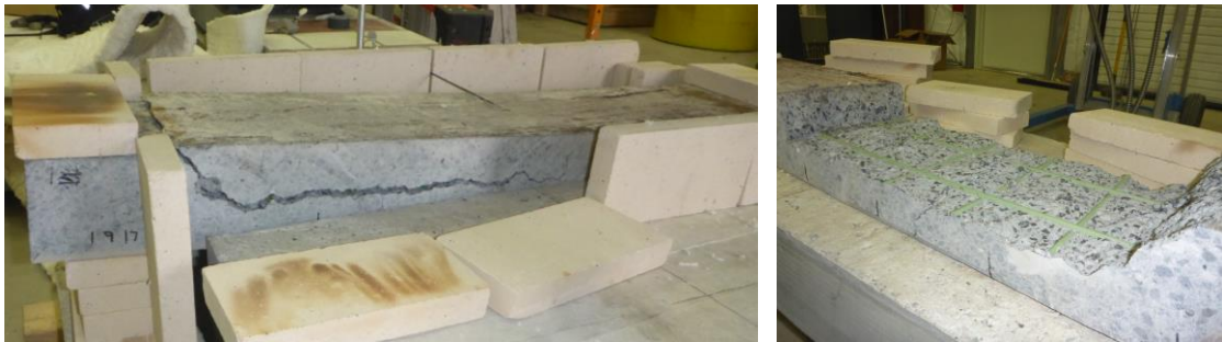
Figure 7.30: Spalled minimally reinforced beam specimen after heating (left), after removal from setup (right)
