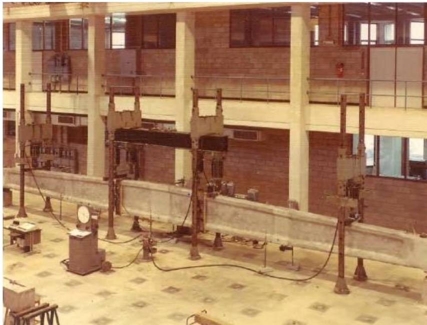
Figure 5.13: Load testing setup for the girder (Reproduced from fib Bulletin 46, page 131 - “Test setup” by Taerwe et al. 2006, with permission from the International Federation for Structural Concrete (fib) [8])
