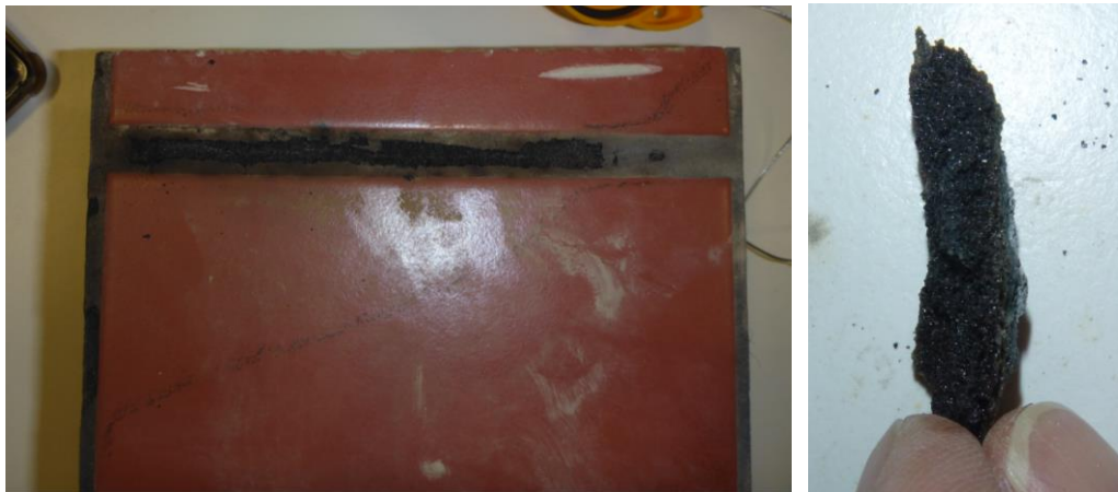
Figure 7.23: Charring of grout material
