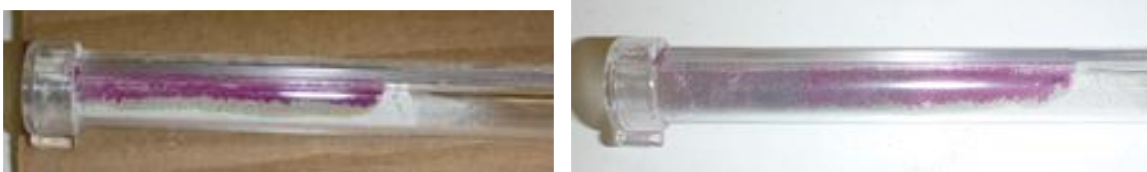
Figure 7.47: Photo of slab Carbontest® tubes from: center of heated zone (left), unheated zone (right)
