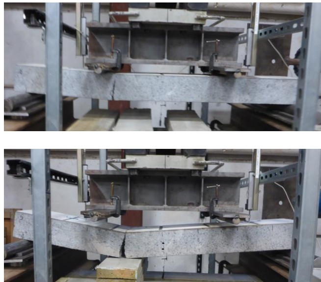
Figure 7.34: Photo of minimally reinforced beam specimens during load testing. Propagation of crack in control specimen during load application (top), after failure of heated specimen (bottom)
