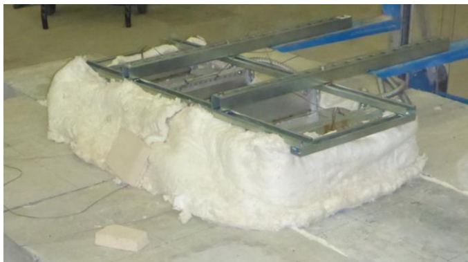
Figure 7.11: Typical Insulation setup. Heating setup before adding any insulation (top), firebrick around heaters (bottom left), insulation around firebrick (bottom right)
