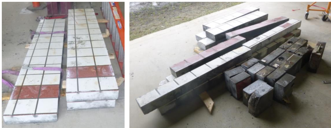
Figure 7.16: Specimens obtained from panel: Three primary beams (left), blocks, smaller beams, and miscellaneous (right)
