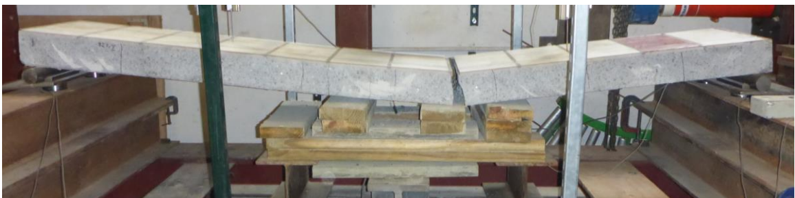
Figure 7.43: Photos of 300°C intact specimen load testing. Multiple flexural cracks in constant moment region during load application (top and middle), after failure (bottom)
