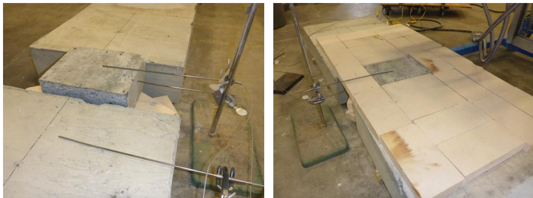
Figure 7.6: Heating of smaller specimen between two throwaway slabs
