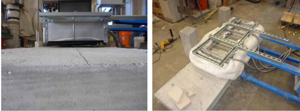
Figure 7.19: Concrete slab heating setup
