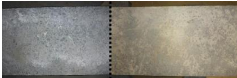
Concrete discoloration at 600°C (1,112°F)
