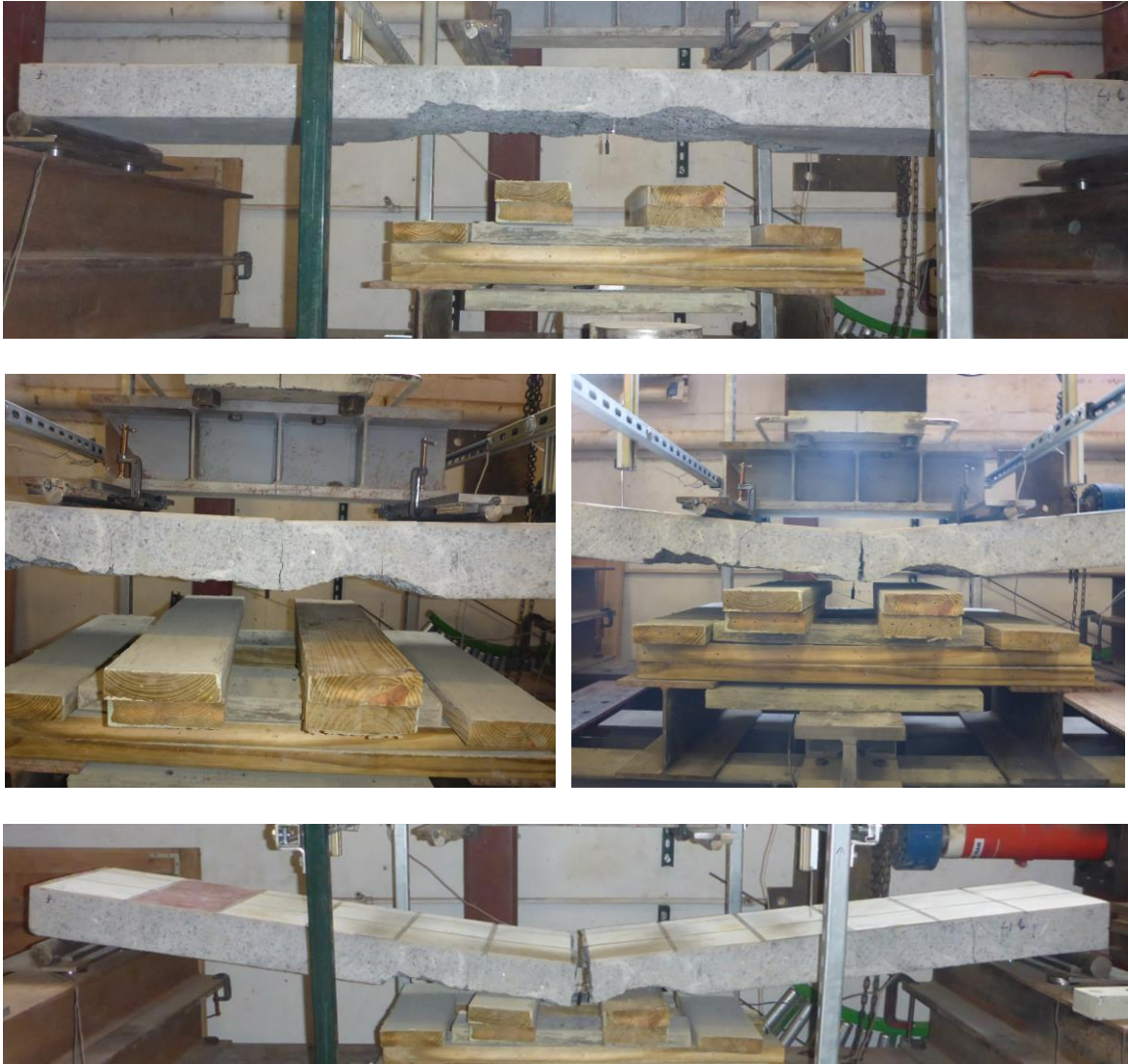
Figure 7.44: Photos of 600°C spalled specimen load testing. Prior to loading (top), propagation of crack during load application (middle), after failure (bottom)
