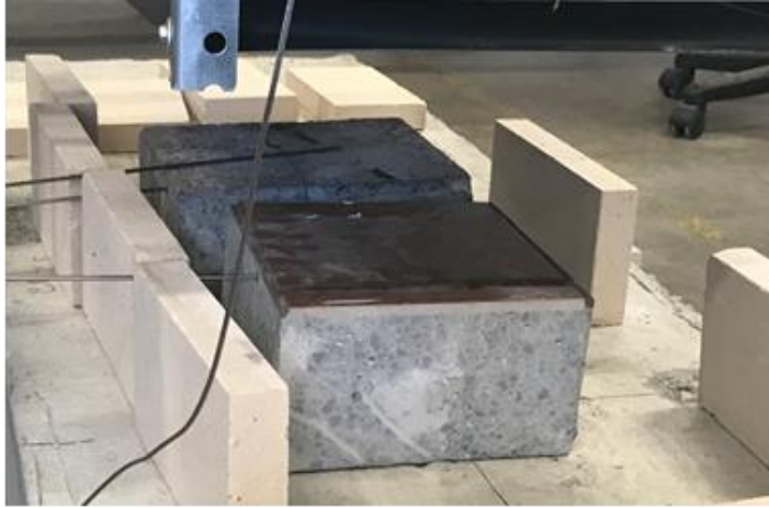
Figure 7.22: Specimens with tile side up (near) and tile side down (far)
