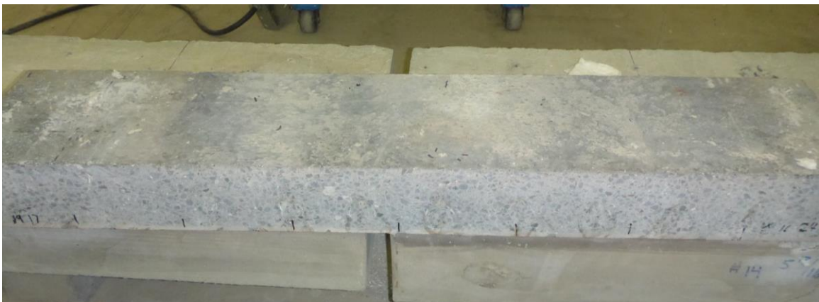
Figure 7.31: Intact minimally reinforced beam specimen after heating
