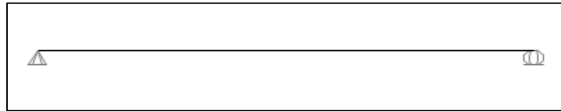
Figure 0.1: Typical Simply Supported 2-D Beam
