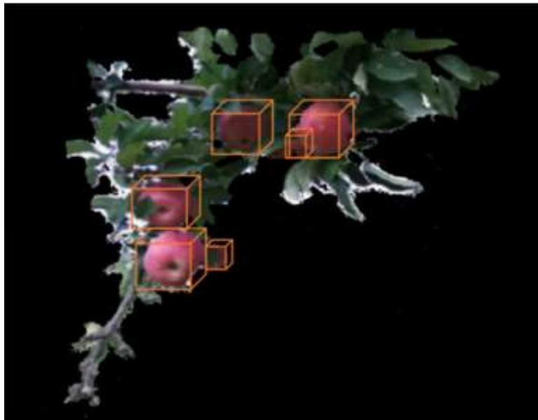
Figure 1.7: The prediction results of apple in 3D bounding box (Tao and Zhou, 2017)
