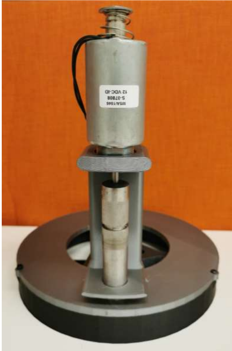
Figure 2.4: The assembled end effector in the real world
