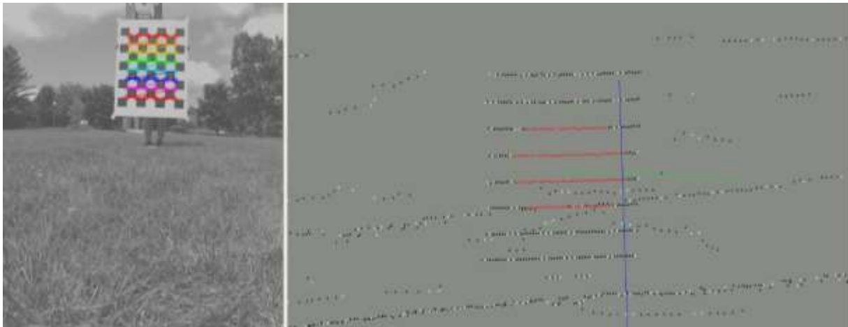
Figure 4.4: One frame of captured chessboard plane in image and 3D point cloud
