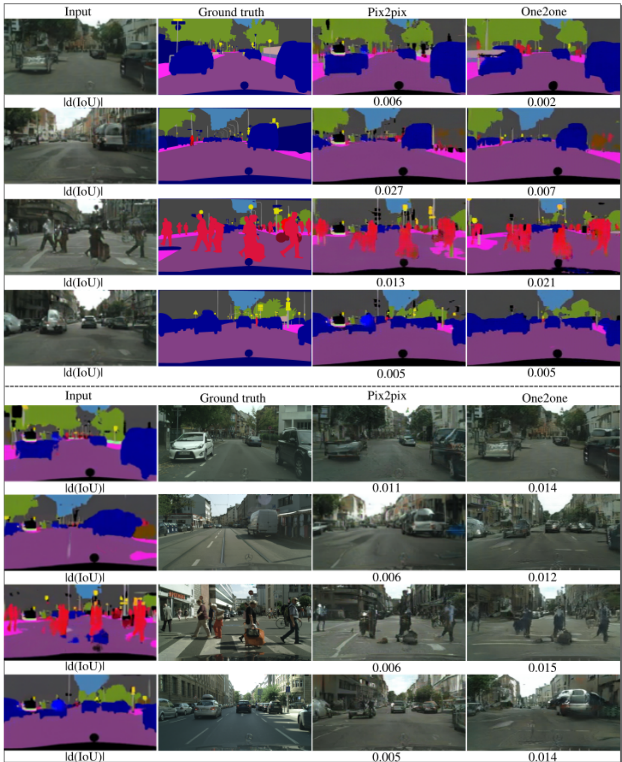
Figure 2.7: Model sensitivity performance of labels \leftrightarrow photo on cityscapes. Upper: photo \rightarrow labels. The input is generated by inputting the groundtruth to pix2pixB. Bottom: labels \rightarrow photo. The input is generated by inputting the groundtruth to pix2pixA.
