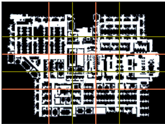
Figure 2.3: The 2d floor plan used to generate random test problems. Here the orange and light green lines shows where obstacles along z axis are placed.
