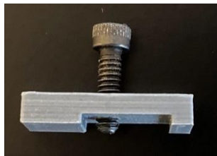
Figure 2.17 Side view of fixture used for holding the front plate in the assembly guide
