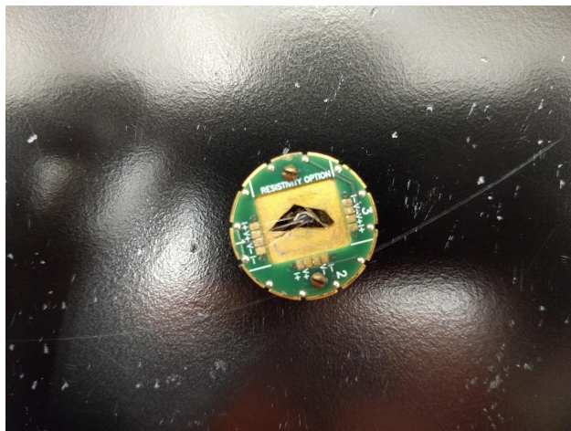
Figure 3.6: Photo of the hexagonal \text{Cu}_{0.82}\text{Mn}_{1.18}\text{As} sample bonded to a resistivity puck for use in PPMS.
