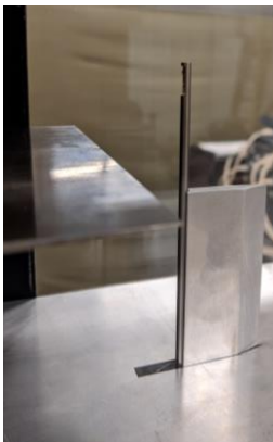
Figure 20. TAT probe mounted in tunnel
