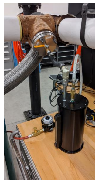
Figure 37. Secondary seeding configuration with Laskin Nozzle seeder
