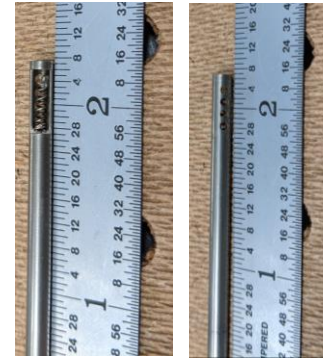
Figure 21. TAT probe front and back showing holes for airflow (with inch ruler for reference)
