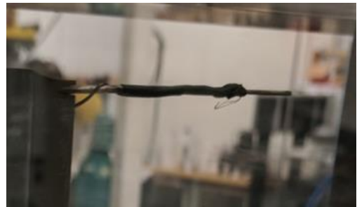
Figure 19. Broken thermocouple on pitot probe
