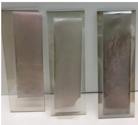
Figure 68. Images of RITC-silica that have been sputter coated for different periods of time (10, 15, and 20 minutes shown left to right).
