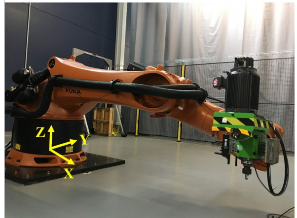
Figure 42 – Test poses used to check cross coupling effects.
