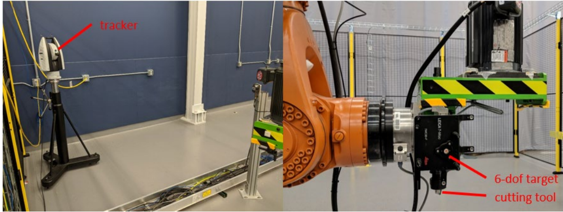
Figure 12 – Left: laser tracker (Leica AT960). Right: 6-dof target (Leica T-Mac) mounted on the end-effector.
