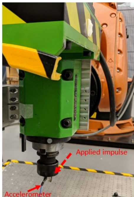
Figure 5 – Robot modal test setup
