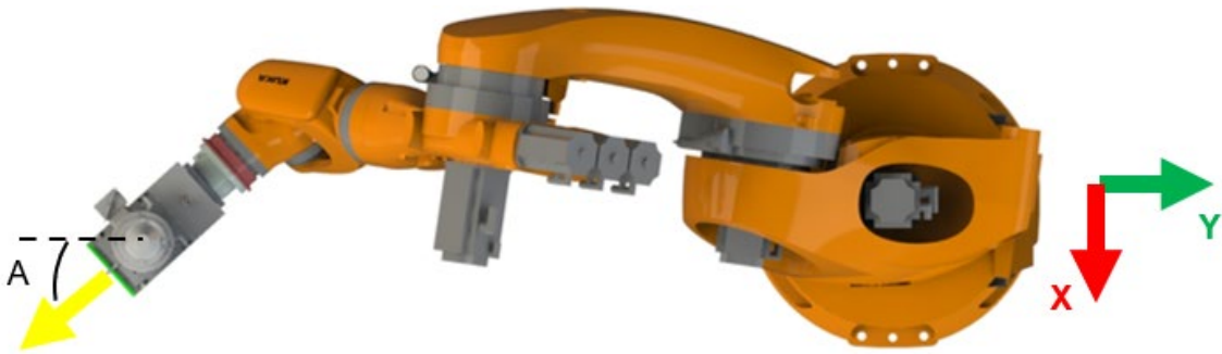
Figure 7 – Optimization of angle “A” about the spindle axis.
