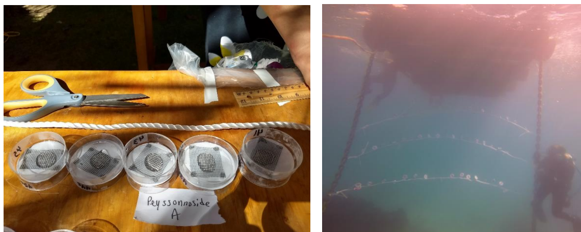
Figure 11. Experimental set-up to evaluate if peyssonoside A ( 7 ) prevented fouling on the surface of phytigel submerged in ocean water for four days. Gels were adhered to window screen (for quantification purposes) that was attached to petri dishes (left image) with paired controls prepared in a similar fashion and attached to the back of the plate containing gel infused with 7 . Plates were deployed under a floating dock off Ono Island, Fiji, for 4 days (right image).
