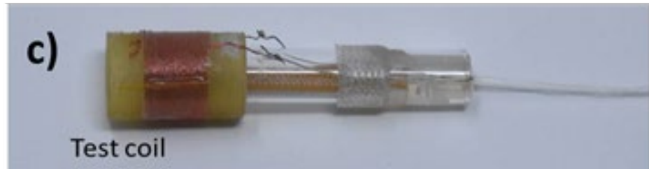
Figure 5-2 Acousto-optic sensor connected to a test coil with a diameter of 8mm and 12 turns.
