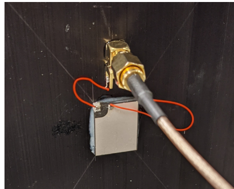
Figure 3.8: Experimental setup for through-metal UPT systems using circular transducers with dimensions (a) 30 x 2.1 mm, (b) 15 x 1 mm (c) 10 x 0.5 mm, and (d) a rectangular transducer with dimensions 20 x 15 x 2.1 mm.
