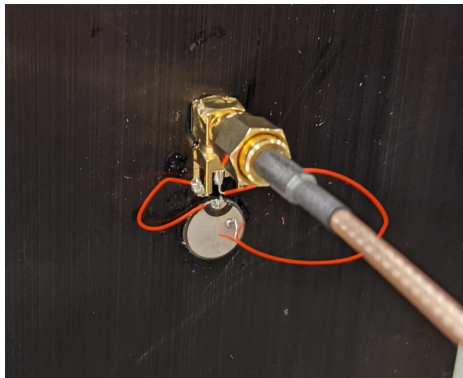
Figure 3.8: Experimental setup for through-metal UPT systems using circular transducers with dimensions (a) 30 x 2.1 mm, (b) 15 x 1 mm (c) 10 x 0.5 mm, and (d) a rectangular transducer with dimensions 20 x 15 x 2.1 mm.
