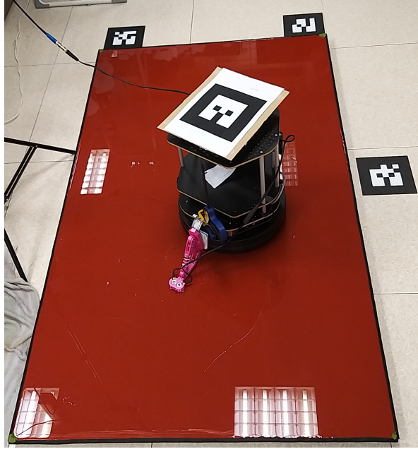
Figure 3.12: Experimental setup. Two co-located pair of transducers fixed on a spring mechanism mounted on the TurtleBot. AR-tags to localize robot's pose relative to the plate's corner.
