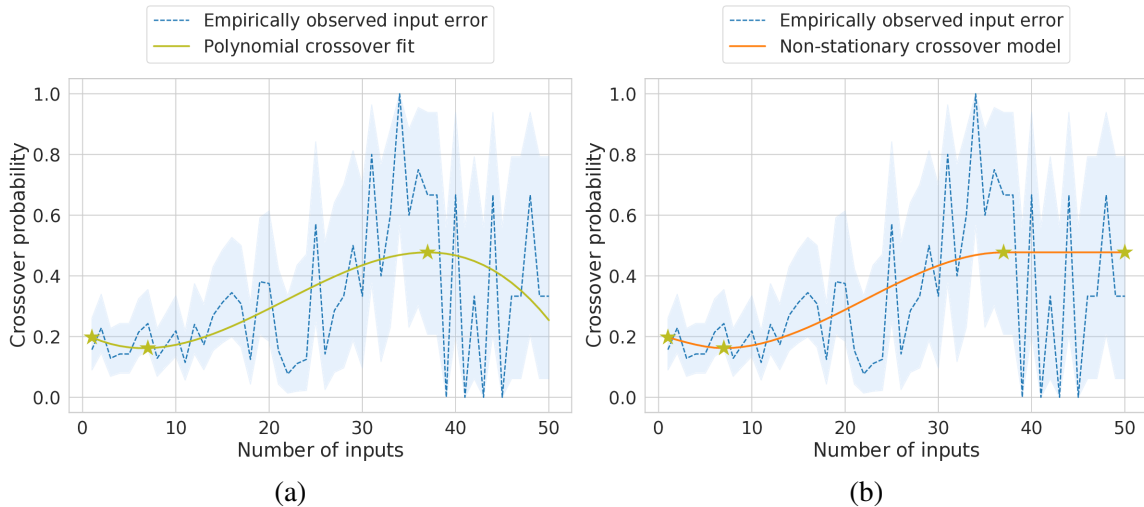
Figure A.7: Modeling a non-stationary input profile from empirical crossover data. a , Least-squares cubic fit to empirical crossover data. The model is highlighted with stars at the first input value, the minimum value, and the maximum value. b , A piecewise cubic Hermite interpolating polynomial (PCHIP) was fit to the first, minimum, and maximum value points from a . We clamped the maximum value to remain fixed until the maximum of 50 inputs, so that the resulting PCHIP error model is non-decreasing. This behavior models the fact that the BCI user may experience fatigue as the number of inputs increases, possibly resulting in non-improving input error statistics after issuing many inputs.
