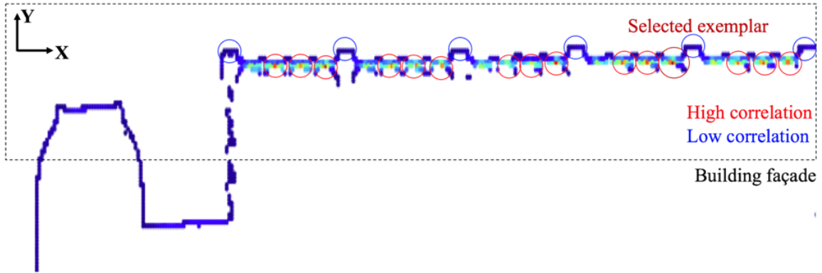
Figure 2.7: Heatmap of feature correlation scores of points along the building façade
