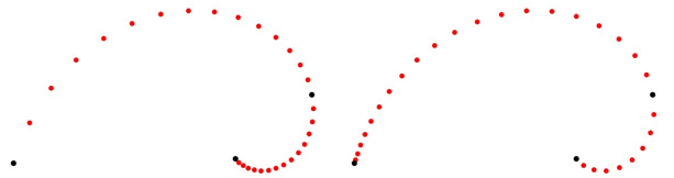
Figure 6: LogSpiral Motion through 3 timed-keyframes (black control points) for b = (a + c)/2 (left) and b = a + 0.7(c - a) (right).
