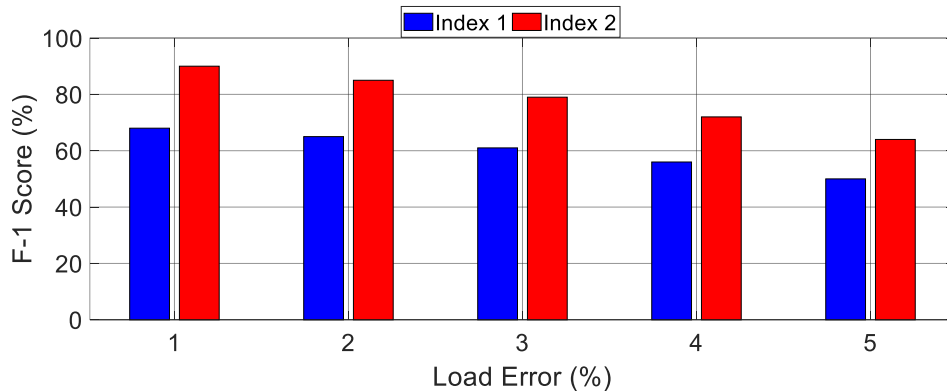
Figure 4.20: The performance of the MaDIoT 2.0 attacks versus the mean error in the New England power grid nodes' power generation/consumption.
