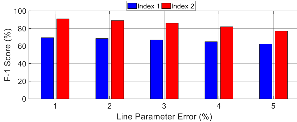
Figure 4.19: The performance of the MaDIoT 2.0 attacks versus the mean error in the New England power grid line parameters.
