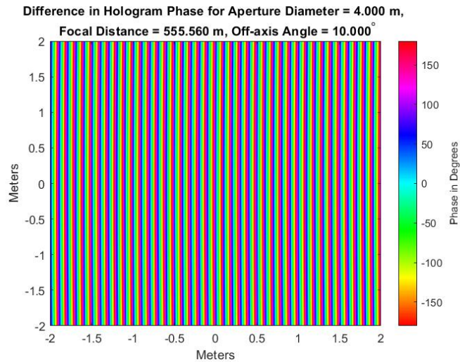
Figure 4.8: Difference in hologram phases for far-field pilot signal and Fresnel-focused pilot signal at 10 degrees off-axis radiation and 555.6m focal distance.
