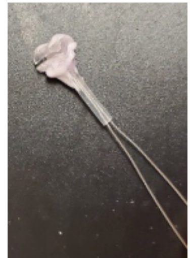
Figure 3: Custom constructed nerve cuff comprised of silicon tubing, wire, and silicon clone.
