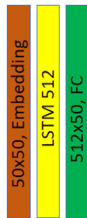
Fig. 17. The LSTM architecture consists of an embedding layer which learns to group input words of similar meaning, an LSTM layer with 512 hidden units for context learning, and then a fully connected layer to predict the next character. The Text8 dataset has 27 unique characters whereas Penn Treebank has 50.
