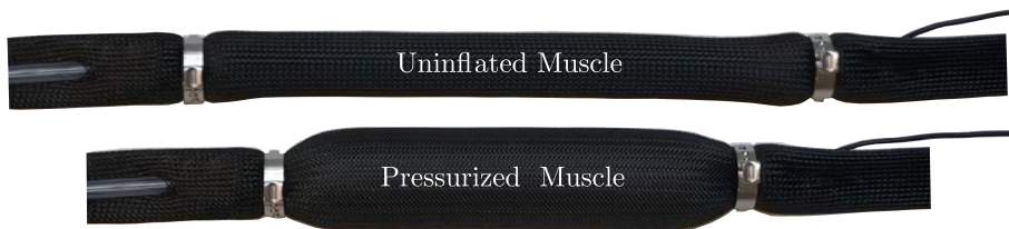
Figure 1.1: Pneumatic artificial muscle: vented muscle at nominal length (top), inflated muscle near max contraction length (bottom).
