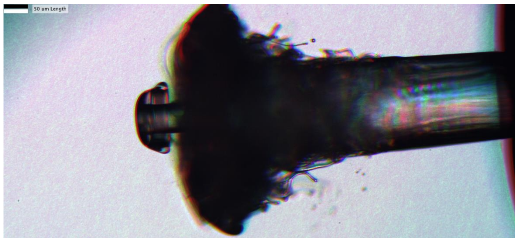
Figure 39: Initial spray formation from phase 2 images. Conditions are 500 bar fuel pressure injecting into STP air. Images are taken 210 \mu\text{s} ASOI and the nozzle diameter is 180 \mu\text{m} .
