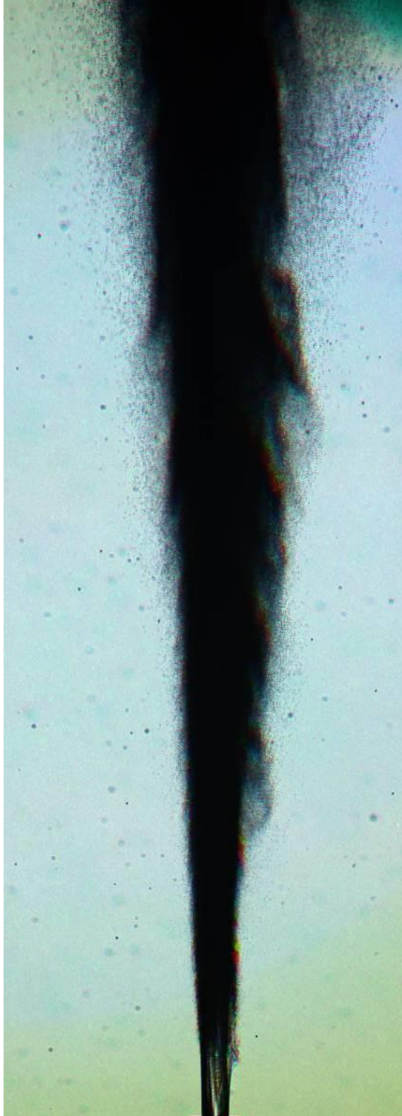
Figure 34: Sample full frame (6000 px wide, cropped height) image from phase 1. Nozzle diameter of 180\ \mu\text{m} , at 500 bar fuel pressure, 6 bar ambient pressure, 1ms ASOI. Nozzle diameter is 180\ \mu\text{m} for scale.
