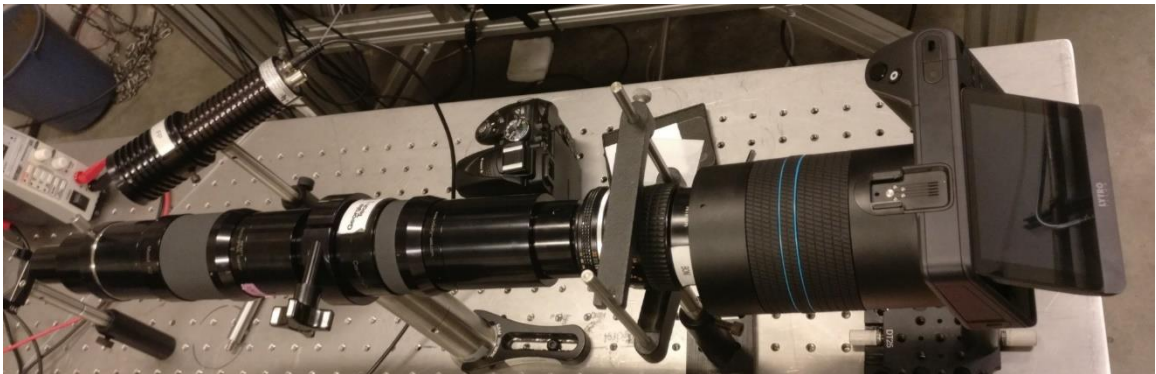
Figure A.1 Early Plenoptic imaging setup using a Lytro Illum, 50mm f/2 relay lens, and infinity K-2S main lens with the 5X CF4 objective.
