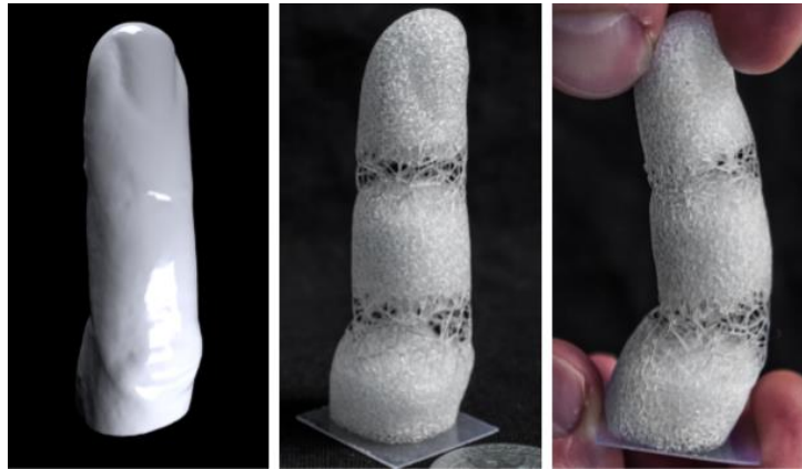
Figure 22 A model of a finger generated using randomized Voronoi foam [68]
