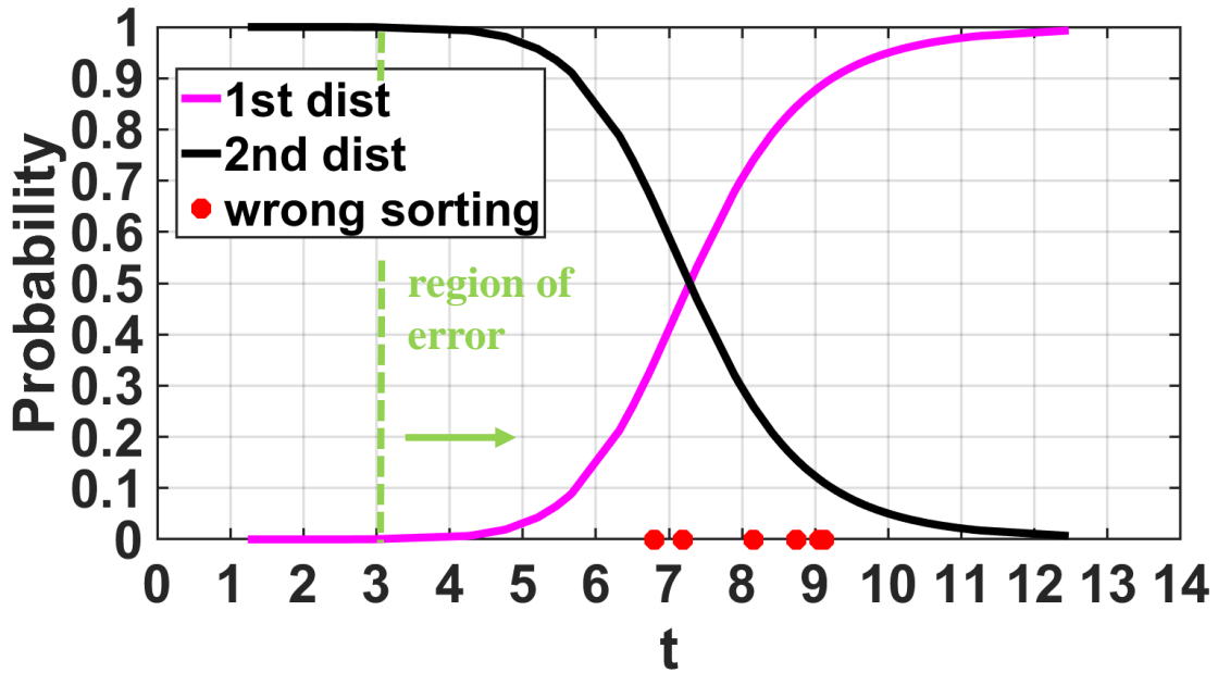
Figure 23 – Sorting accuracy of 93.0% for FEOL TDDB (1 st dist.) vs. EM failure (2 nd dist.) in 14nm FinFET ring oscillators for a sample size of 100.
