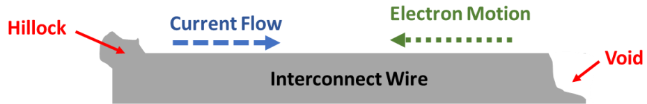
Figure 14 – Formation of hillock and void resulting from electromigration.
