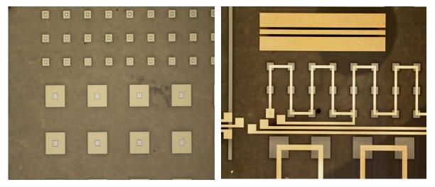
The transferred SiO<sub>2</sub>-reconstituted-tier after removing the silicon handle layer
