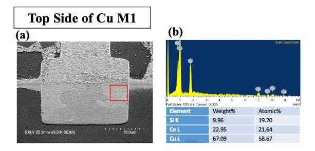
Figure 27 (a) SEM characterize of the silver deposit on the bonding-pad after ALD Co deposition for 1,000 cycles, (b) EDS reading of the red square area [92]
