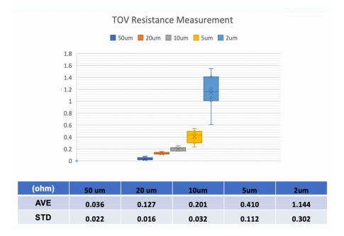
Figure 41 TOV resistance measurement with different diameters
