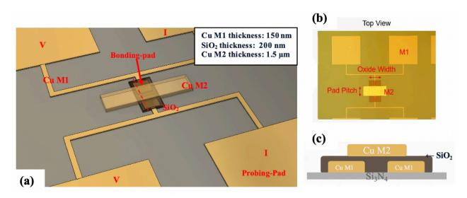
Figure 23 Co ALD Test-Bed Final Design (a) 3D CAD model, (b) Top view, (c) Side view [92]
