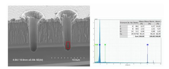
Figure 36 Through-oxide-via with Cu
