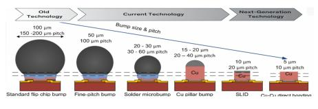
Figure 10 Trend of I/O bonding (Adapted from [11])
