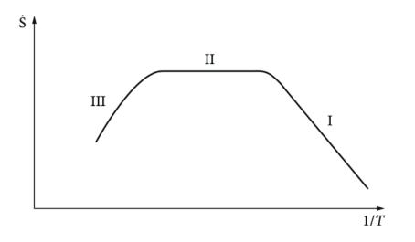
Figure 16 Three different temperature regimes for CVD
