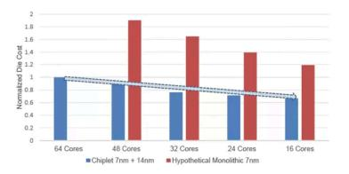
Figure 4 Comparison of normalized cost reduction for homogeneous and heterogeneous integration [13]
