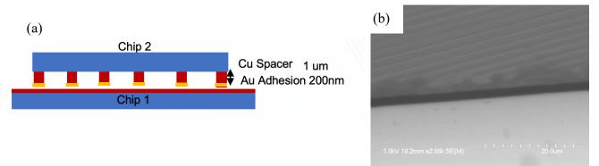
Figure 42 (a) Design schematic for ALD gap-filling testbed, (b) Preliminary fabrication result on the side view
