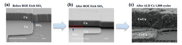
Figure 25 SEM side-view of testbed (a) Before BOE etch SiO<sub>2</sub> sacrificial layer, (b) After BOE etch SiO<sub>2</sub> to create the gap, (c) After 1000 cycles of Co ALD deposition [92]
