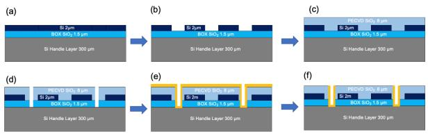
Figure 33 Fabrication steps for SiO<sub>2</sub>-reconstituted-tier
