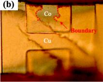
Figure 26 Optical Microscope Image of Bonding-Pads After Peel Off Cu M2 layer (a) Top Side of Cu M1, (b)Bottom Side of Cu M2 [92] was peeled off. EDS characterization was also used to characterize surface chemistry and confirm the deposition of Co on the peeled pads, as shown in Figure 27 (b).
