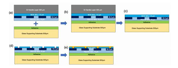
Figure 37 SiO<sub>2</sub>-reconstituted-tier transfer by handle layer removal
