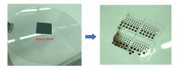
Figure 38 (a) The SiO<sub>2</sub>-reconstituted-tier mounted onto the glass supporting substrate, (b)
