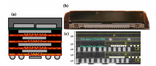
Figure 14 TSMC 3D Fan-Out Wafer Level Package (a) The concept, (b) Optical microscope cross-section image, (c) SEM cross-section image [65]
