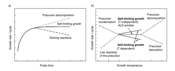
Figure 18(a) ALD growth rate and pulse time relation, (b) ALD growth rate and growth temperature relation [70]
