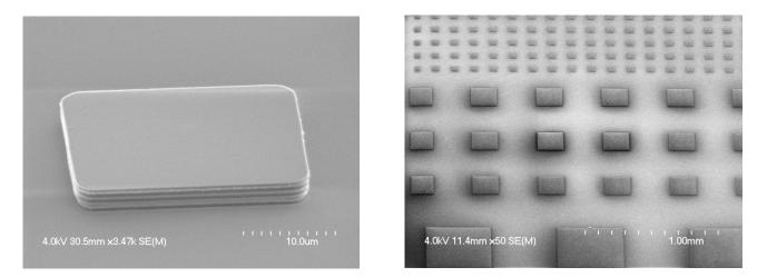
Figure 34 (a) Emulated chiplets from SOI device layer, (b) Multiple sizes of emulated chiplets
