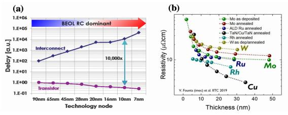
Figure 3 (a) Relationship between interconnect RC delay and the technology node, (b) Cu resistivity increases with scaling [8] [9]
