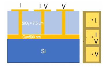
Figure 40 TOV resistance measurement design (a) Schematic side view, (b) Top view
