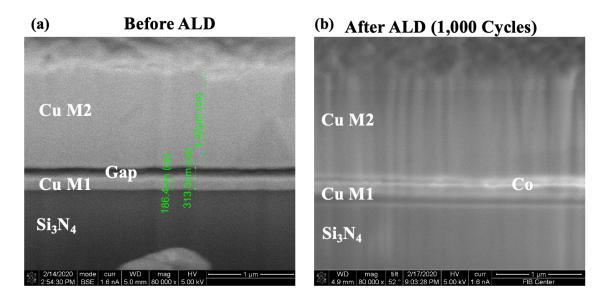
Figure 28 FIB Cross-Section across the bonding-pads (a) Before ALD, (b) After ALD Co Deposition 1,000 cycles [92]
