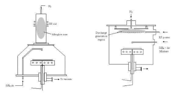
Figure 19 Inductive coupled PECVD and capacitive coupled PECVD [70]
