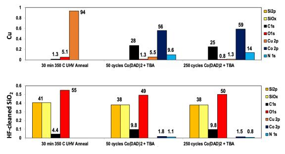
Figure 29 XPS of Cu and SiO2 during different cycles
