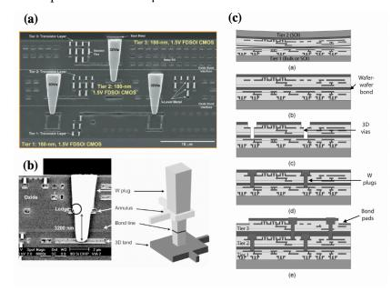
Figure 13 Lincoln Lab 3D Circuit Integration Technology [44] (a) Three tiers of SOI oxide layer, (b) Close-up view of the via, (c) Process schematics
