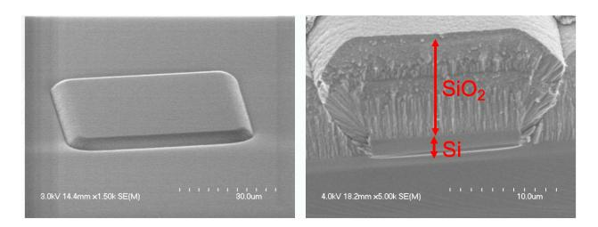
Figure 35 (a) top view of chiplet encapsulate by 8  $\mu$ m SiO<sub>2</sub>, (b) cross-section of chiplet encapsulate by 8  $\mu$ m SiO<sub>2</sub>
