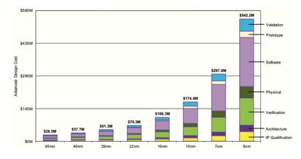
Figure 2 Exponential increase for design cost at advanced nodes [6]
