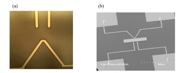
Figure 43(a) Smaller pad size testbed, (b) Contact resistance measurement testbed
