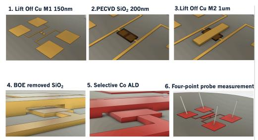
Figure 24 Fabrication and Experiment Steps [92]
