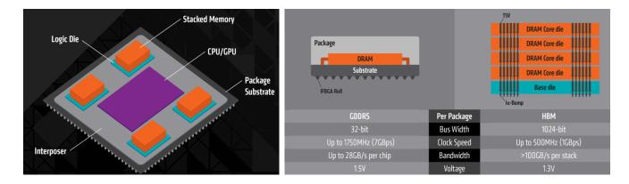
Figure 5 AMD HBM schematic and performance comparison [17]
