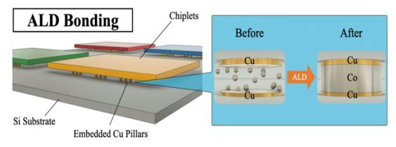
Figure 21. ALD bonding schematic [92]
