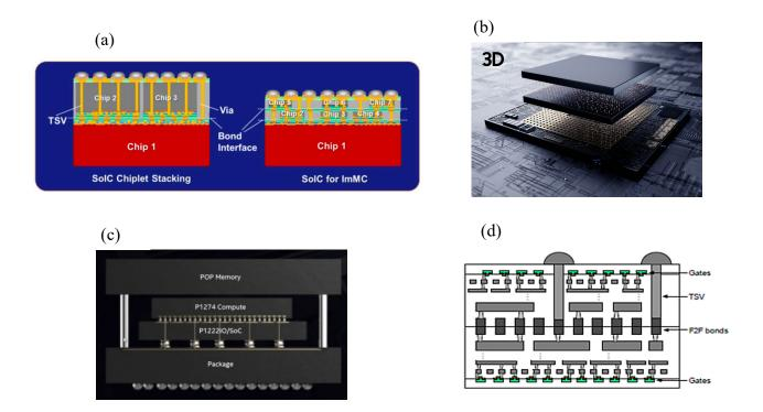
Figure 7 (a) TSMC SoIC [19], (b) Samsung X-Cube [20], (c) Intel Foveros [24], (d) GlobalFoundries HWB [22]
