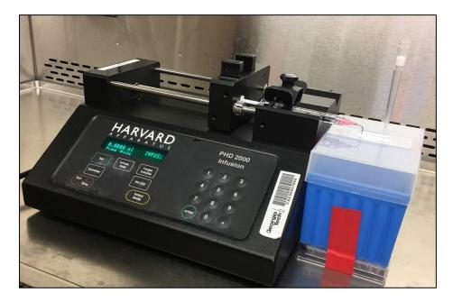
**Figure A. 5: Sterile microfluidic device setup in BSC.** Example setup for sterile microfluidic device operation in a biosafety cabinet. This setup utilizes a needle attached directly to the syringe without tubing to minimize void volume and reagent waste. The device is elevated so that the needle can plug directly into the inlet without tubing. A barrier pipette tip is plugged into the outlet to collect the cell sample and minimize contamination risk.
