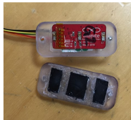
Figure 2.5. Conductive Silicone Electrode Contacts. The electrode contacts in this picture are made of conductive silicone so that they are pliable, conformal and provide a more stable interface to the skin.
