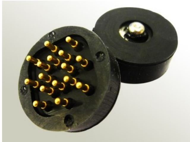
Figure 2.3. Spring Loaded Polymer Electrodes [62]. These electrodes are particularly useful for EEG acquisition as they allow for good contact with the scalp, are compliant and water/oil resistant.
