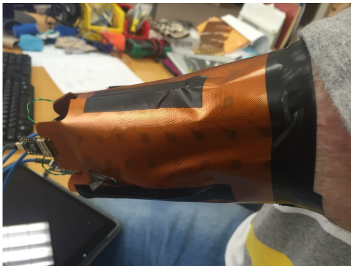
Figure 4.2. Hardware for HD EMG. The image on top shows a HD array used for HD EMG acquisition. The electrode array is made of out Flex PCB and has 128 contact points. Each array is separated into 4 different 32 channel arrays. Each array connects to a 32 channel amplifier board and ultimately leads to a processor that simultaneously processes all 128 channels of data. The figures on the bottom show the array being used on a trans-humeral amputee and on an able bodied individual.
