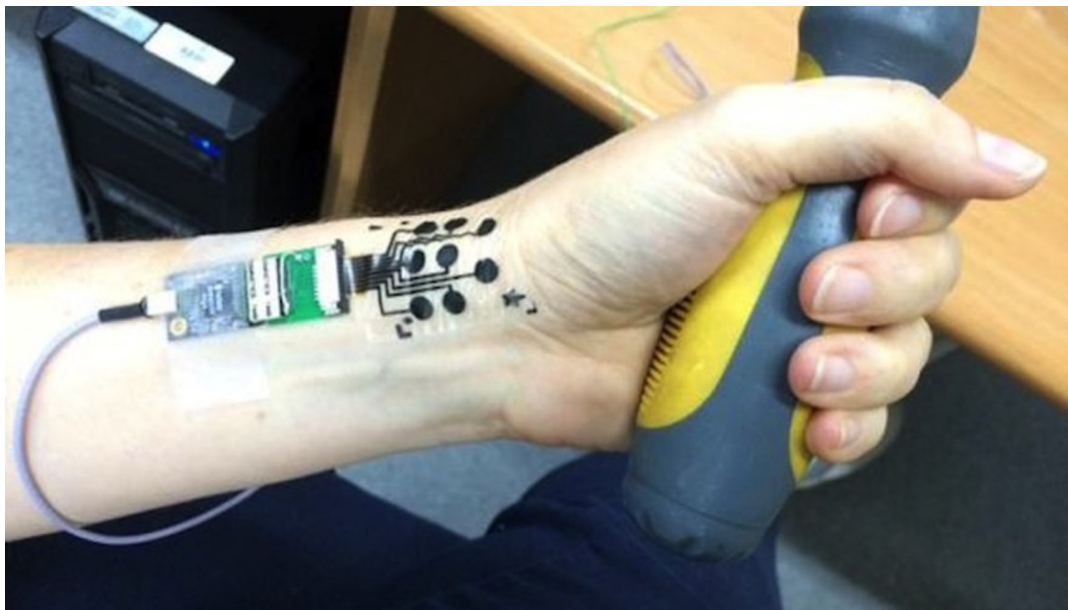
Figure 2.4. Polymer based Electronic Tattoo [60]. The concept of tattoo based wearable electronics is becoming sought after technology due to the stability it provides to the skin electrode interface. However, long term use of these circuits is not feasible currently and remains the biggest hurdle towards their commercial adoption.
