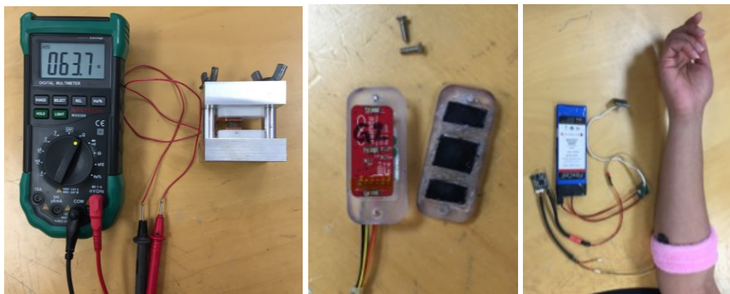
Figure 3.3.a. The apparatus for conductivity measurements. The material is placed between the metal plates of the mechanical contraption, which is held at a constant spacing using spacers. The wires leading out of the measurement rig are connected to the digital multimeter and DC resistance is measured. The same is used with the Intan system for complex impedance measurements.
