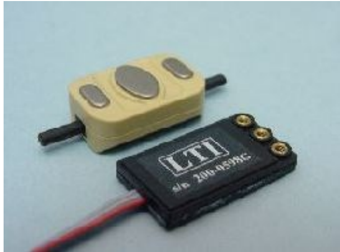
Figure 1.3: Dry EMG electrodes [8]. Dry EMG electrodes are currently the industry standard for myoelectric prosthesis, EMG acquisition. Numerous companies like Ottobock, LTI, and CoAPT commercialize different dry electrode technologies such as analog electrodes, digital electrodes and remote electrodes.
