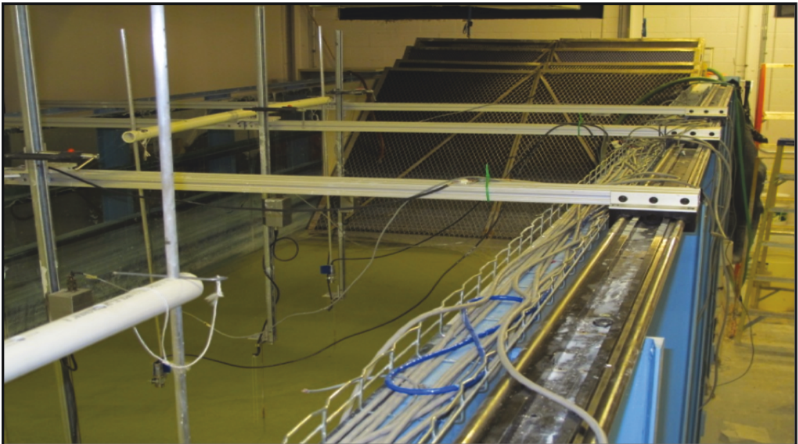
Figure 3.4: The wave tank, beach end with the cages layers with wave absorbing material.
