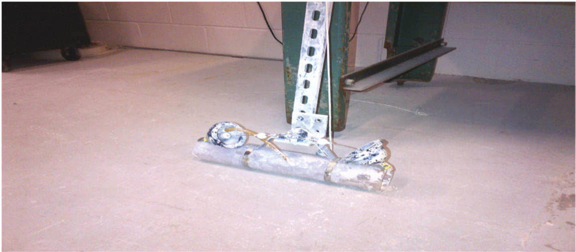
Figure 4.2: The density sampler used to collect mud from the bottom of the tank.
