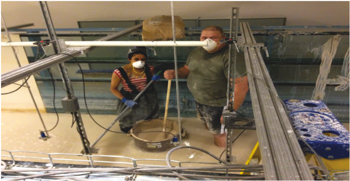
Figure 4.3: The mud is mixed manually by using a 60 gallons barrel to create a well water-mud mixture.
