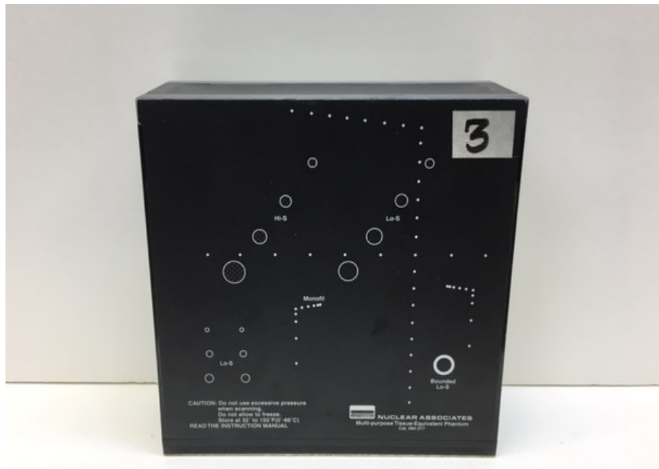
Figure 6.11 Planar general ultrasound phantom used in virtual fixtures experiments. Next steps will aim at imaging more anatomically accurate phantoms.
