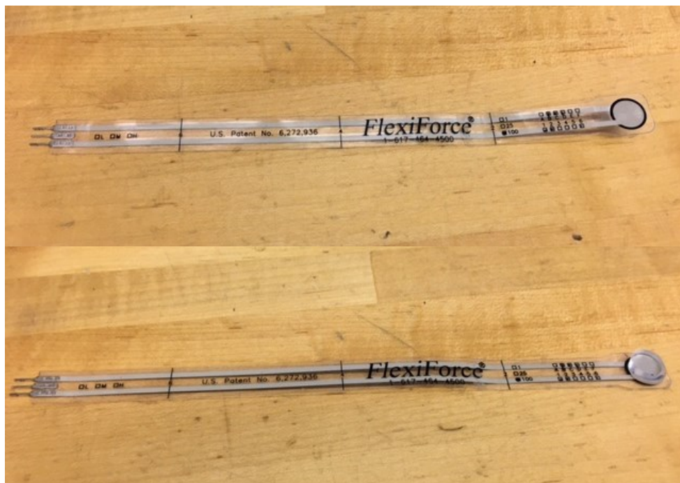
Figure 4.2 Modification of FlexiForce A201 (Top) Sensor without modification. (Bottom) Sensor with force-distributing "puck" adhered to sensing area
