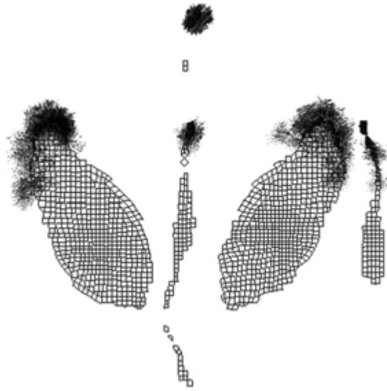
Figure 14: The UV map for the adipose-derived stem cell. Here, the grid-like structures represent the model polygons. Most of the map is white (opaque), while black texture is painted where the cell will be transparent.
