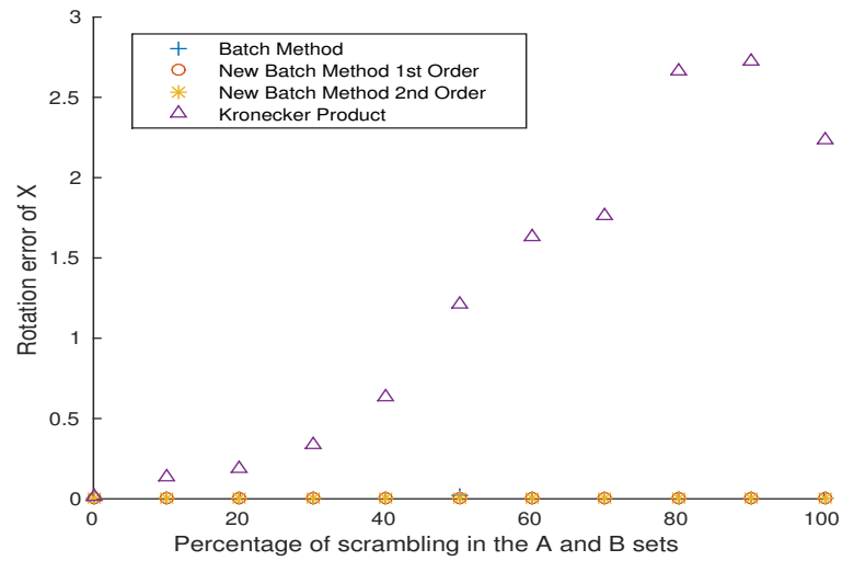
Figure 5.5: Rotation error vs. percentage of scrambling in \{A_i\} and \{B_j\} for the Batch, Batch1, Batch2 and Kronecker product methods where \{B_i\} is generated using Eq. (5.21). Results of Batch method are overlapped by Batch1 & Batch2 and a close look can be found in Fig. (5.7)
