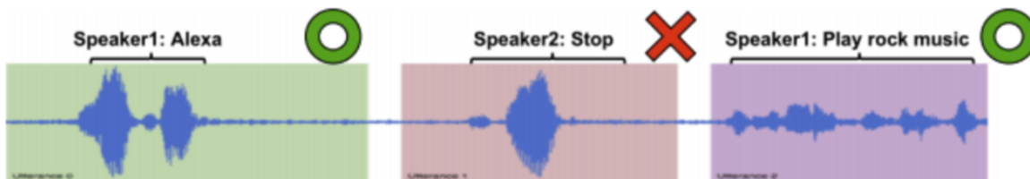
Figure 5.1: An illustration of anchored speech recognition. We would like to suppress speech from Speaker 2 and only recognize that from Speaker 1, because it is Speaker 1 who says “Alexa” to the device.
