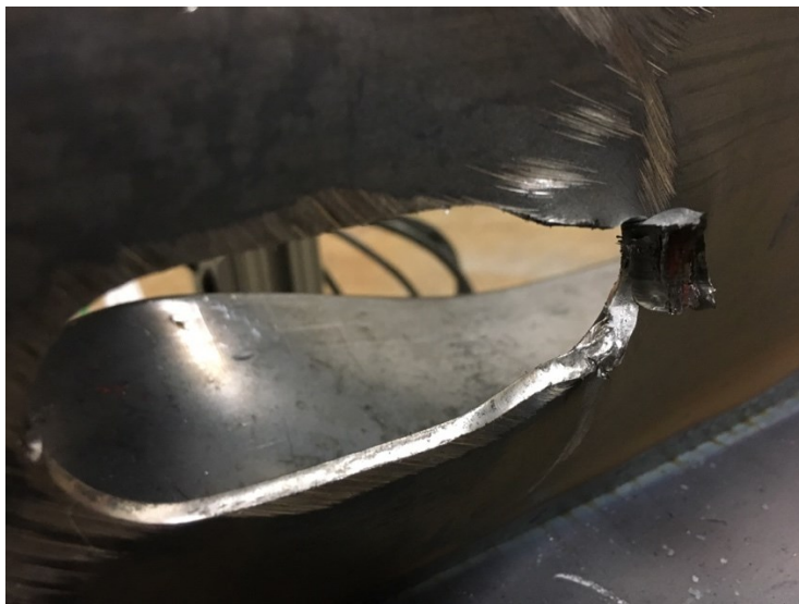
Figure 7-14. Typical web tearing deformation at the hillside washer nipple bearing point (W1 test shown)
