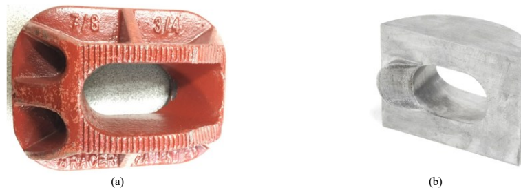
Figure 7-3. Hillside washer types reported in the survey: (a) hardened steel with an oversized bearing surface and nipple for engaging web edge; and (b) an aluminum hillside washer.
