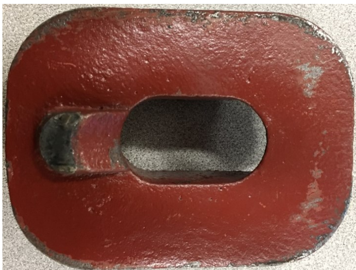
Figure 7-15. Hillside washer nipple bearing failure (C3 test shown)
