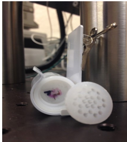
Figure 21 Ogawa badge sampler with responsive device mounted inside.
