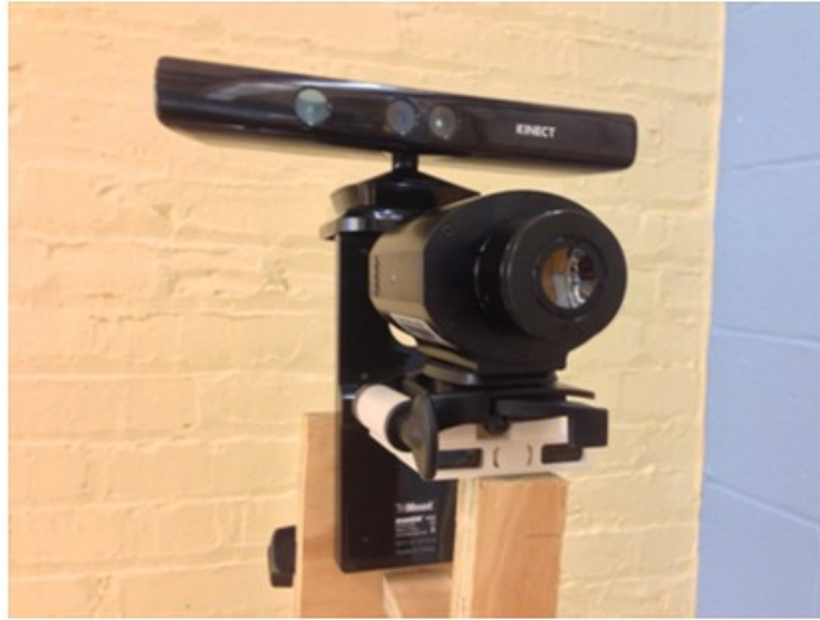
Figure 5.1 The 3D infrared imaging system developed at the Heat Transfer Lab of JHU combining the Kinect imager (top) and the infrared camera (bottom).
