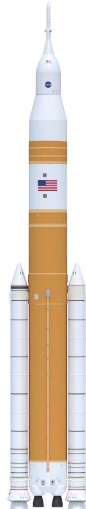
Figure 8 – This configuration of the SLS, with the Exploration Upper Stage, will provide in-space propulsion to send astronauts in NASA's Orion spacecraft and heavy cargo on a precise trajectory to the Moon. Image credit: NASA.
