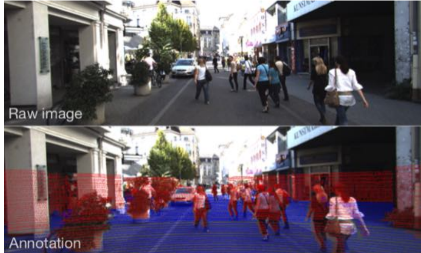
Figure 1.1. An illustration of the 3D roadplane detection problem. The raw image is from KITTY-CITY-71 [40]. We annotate the frame such that the (noisy) inlier points associated with the roadplane are in blue and outlier points are in red. The goal is to identify the underlying roadplane.
