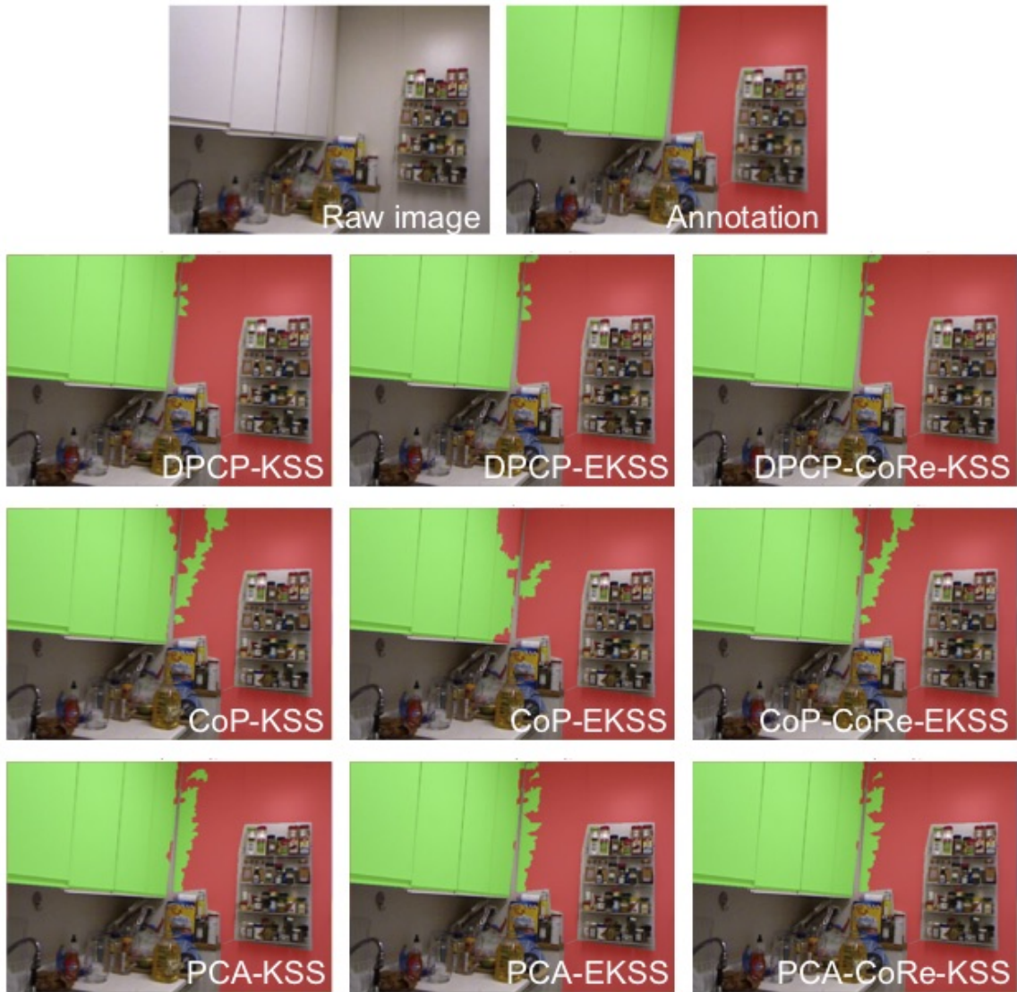
Figure 5.3. Visualization of various approaches in clustering two hyperplanes from a 3D point cloud of image 55 in NYUdepthV2.
