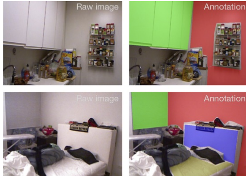
Figure 1.2. An illustration of the 3D plane clustering from an indoor scene. The raw images are from NYUdepthV2 [92]. We annotate the frames such that the (noisy) inlier points associated with each plane are in the same color. The goal is to learn the underlying plane arrangement given the 3D point cloud data.
