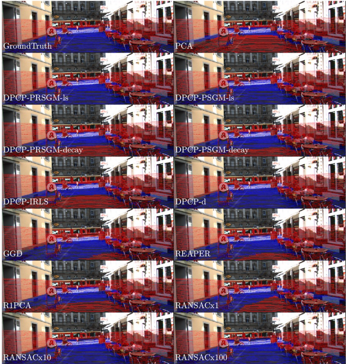
Figure 4.8. Projections of 3D point clouds for frame 881 of KITTY-CITY-71 onto the image, with inliers in blue and outliers in red.
