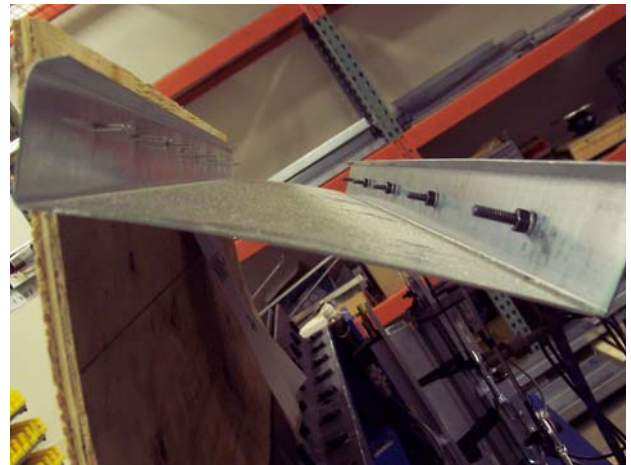
#6 @ 6 in. o.c. with 800S200-54 joist
