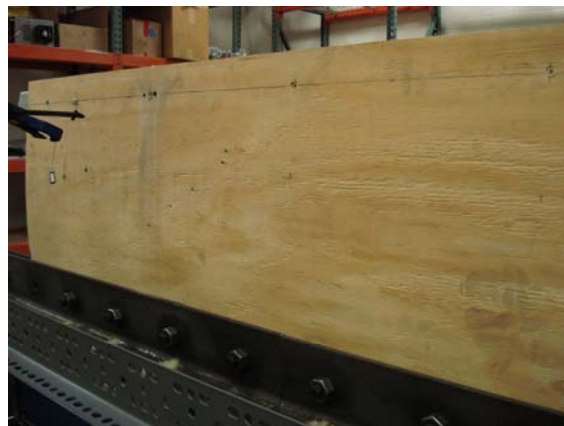
Figure 10 Detail of test setup from behind, cantilever length is taken from the tip of the clamping angles to the fastener line (12 in. or 24 in. from the tip of the angles)
