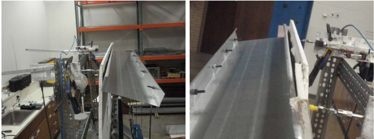
(a) large separation between joist and gypsum board shown for an 800S200-54 joist with gypsum board, L = 12 in., and #10 fasteners @ 12 in. (6-GYP-24-10-12-01, 6-800S200_54_33)
