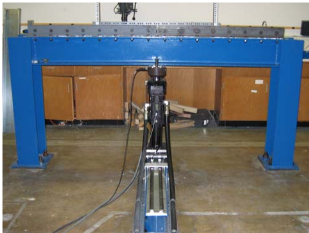
(a) front view of testing rig, angles spaced with holes 6 in. o.c. are attached to specimen for fixed conditions
