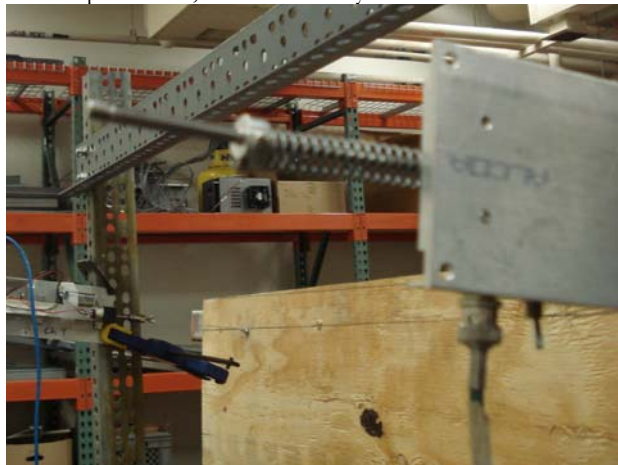
(c) stiff spring added to transducer, spring found to be overly stiff and was used on only two tests, see Table 7
