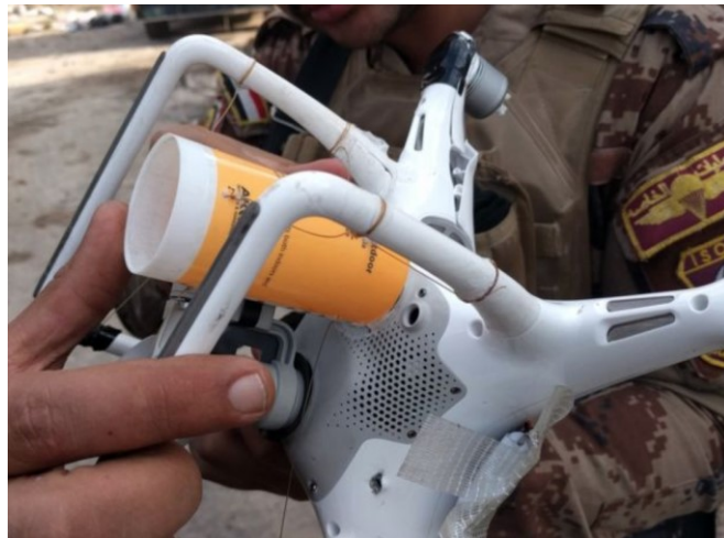
Figure 3: Custom-made COTS drone with a cup mounted to the bottom 43
