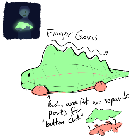
Figure 3.18: An example design from the iterative design process followed for the design of interactive device (Credits: Erica Huang)
