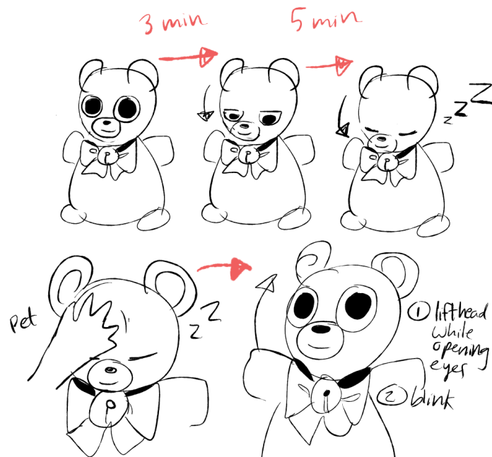
Figure 3.7: An example sketch from the iterative design process that shows the robot behaviour design for idle state (Credits: Erica Huang)
