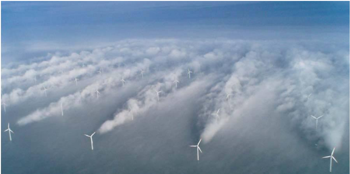
Figure 1.4: Wind turbine wakes in Horns Rev wind farm visualized by the formation of fog. Figure is reproduced from Hasager et al. 6 and licensed under CC BY 3.0.
