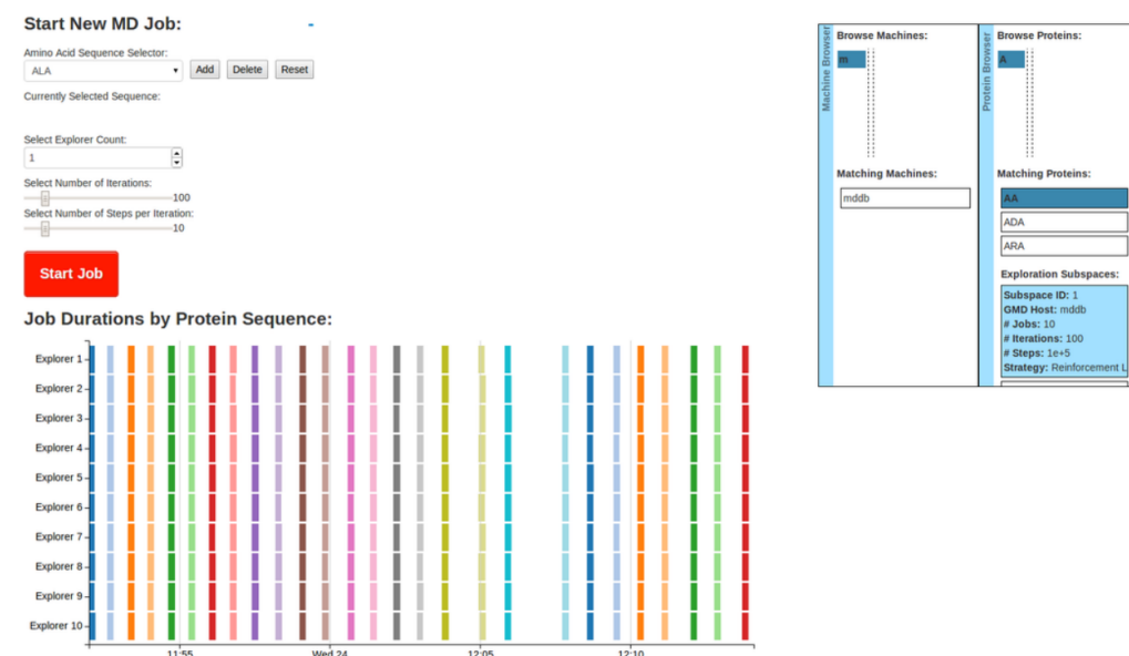
Figure 2.9: Web interface allows users to easily start new protein simulations. Ongoing and past simulations' progress and hardware impact monitored in real-time. Colored bars represent protein simulation execution. Between each iteration, adaptive control or reinforcement learning module assesses best way to guide simulation
