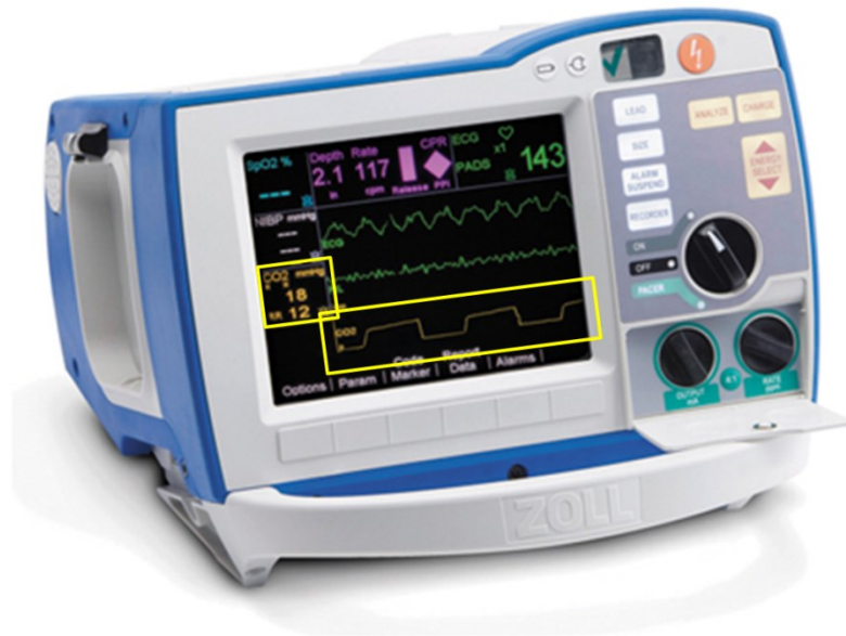
Figure 3.4. ZOLL R Series Plus defibrillator display of Capnostat5 ETCO 2 sensor (boxed in yellow). Maximum amplitude and respiratory rate shown numerically on left sidebar, and ETCO 2 waveform displayed bottom center. (Adapted from ZOLL.com)
