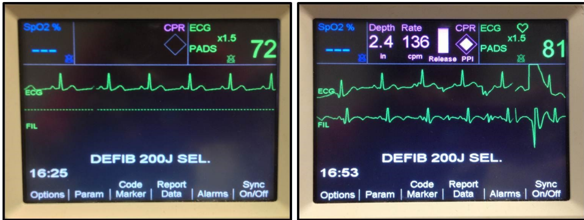
Figure 2.7. ZOLL R-Series defibrillator screen when attached to a rhythm generator (left) and when connected via pads to this device.
