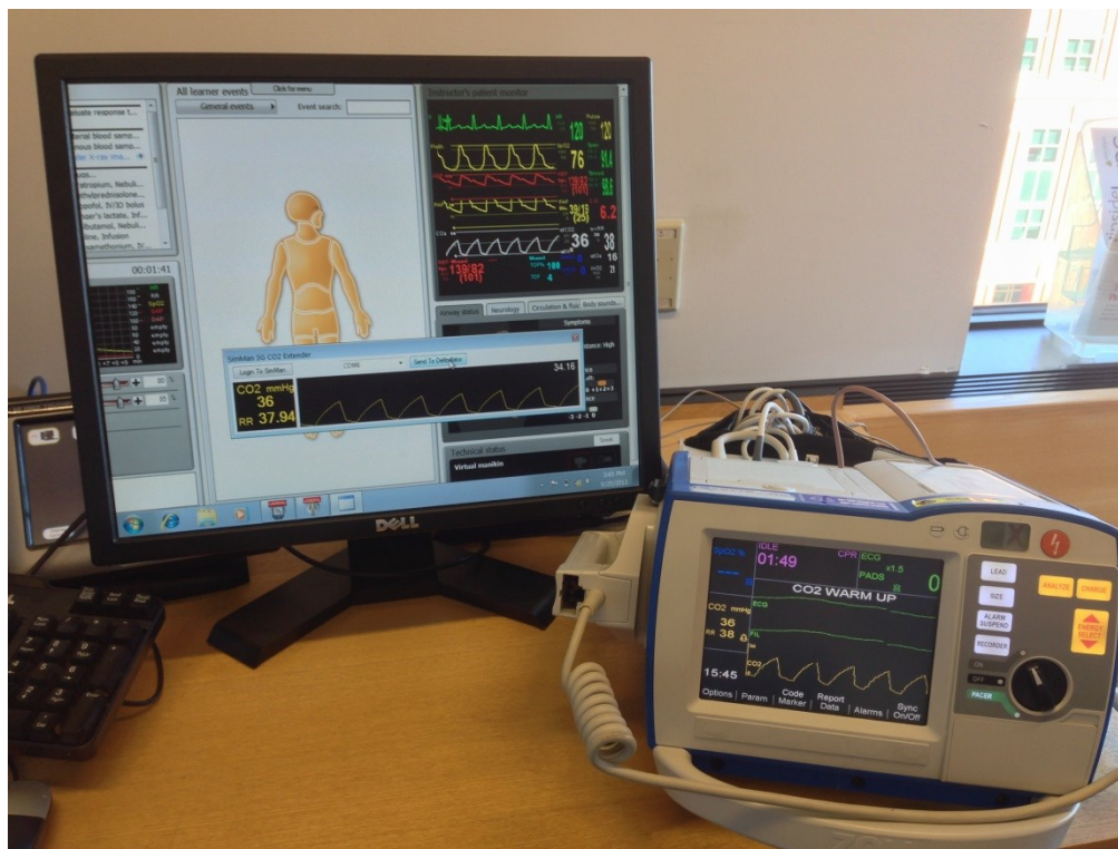
Figure 3.11. ETCO 2 waveform values collected from SimMan3G waveform generation software and formatted for transfer to ZOLL R Series defibrillator.
