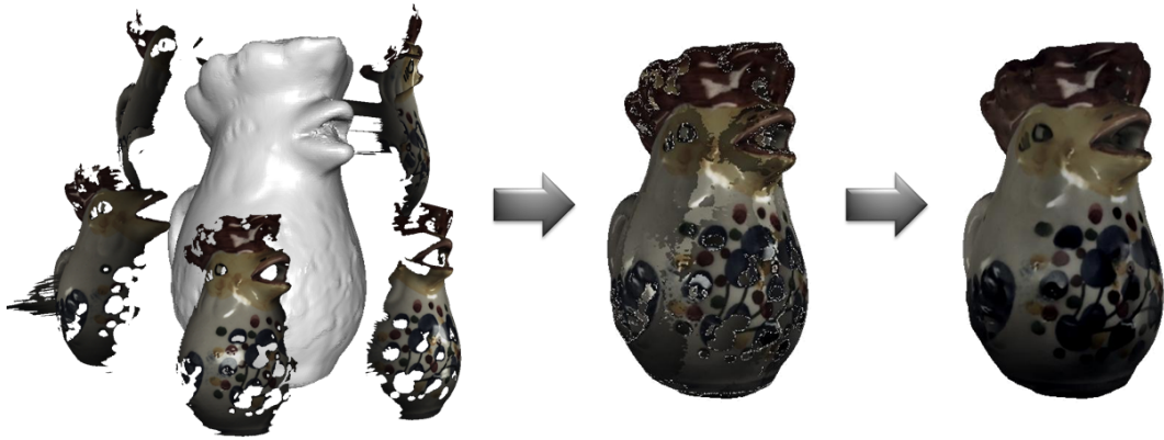
Figure 1.2: Color reconstruction of the rooster model from 3D scans ( left ). Due to the lighting variation across scans, directly pulling color values from the closest scans results in visible discontinuities at scan transitions ( middle ). Taking color gradients from the closest scans instead and solving the Poisson equation gives a seamless stitching result ( right ).
