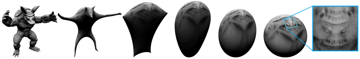
Figure 6.8: Conformalized Mean-Curvature Flow applied to the Armadillo Man. From left to right, we show the 0th, 1st, 3rd, 5th, 10th and 30th steps of the flow. Note that the flow conformally evolves the mesh to a sphere (right).
