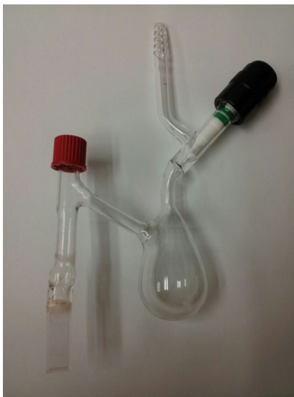
Figure A3.1. Schlenk cuvette (5 mm pathlength) used for air and water-free solution preparation. The barbed inlet (top) connects to a schlenk line (vacuum or N_2 ); the red cap utilizes a PTFE coated septum to allow for addition or removal of solutions. Solutions are deaerated by Freeze-Pump-Thaw in the pear-shaped flask and are then transferred into the cuvette by tilting the flask.
