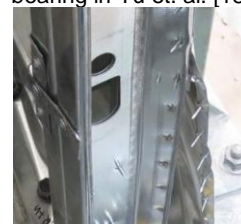
(e) Pull-out in Rizk et. al. [5]
