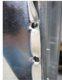
(a) Pull-through in Rizk et. al. [5]
