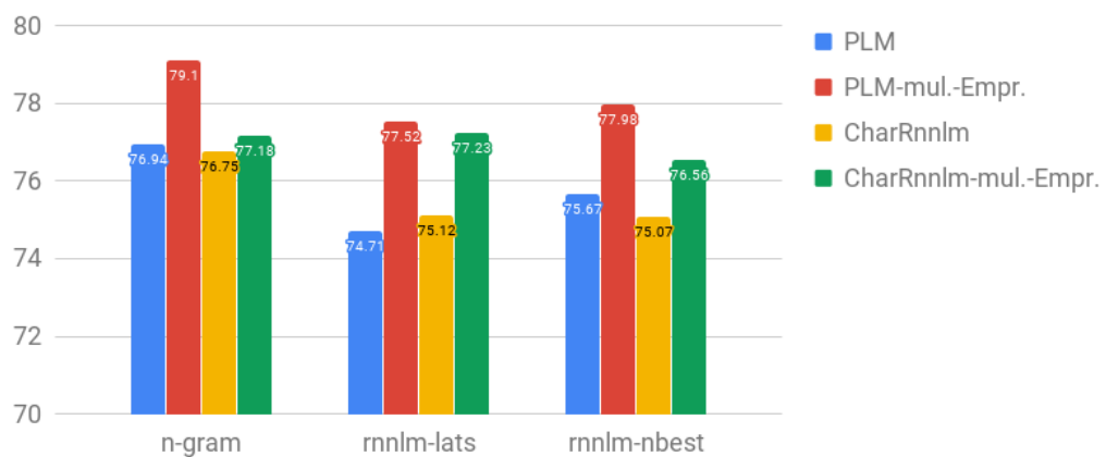
Figure 3.44: Impact of different estimation schemes of OOV unigram probabilities on OOV WER, on "Test-other" subset
