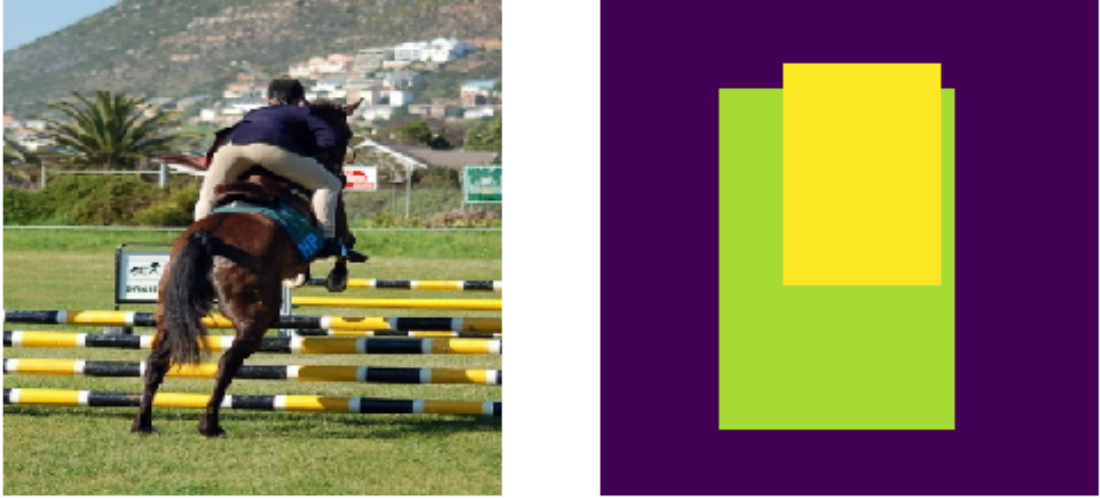
Figure 4.5. Example of weak (pseudo) segmentation ground-truth. Left: Input image with a size of 300 \times 300 pixels, with a person and a horse on the image. Right: Weak segmentation ground-truth for the left image, with a size of 38 \times 38 ; the pixels locate inside both the person and the horse bounding-boxes will be assigned to person class since its bounding-box is smaller.
