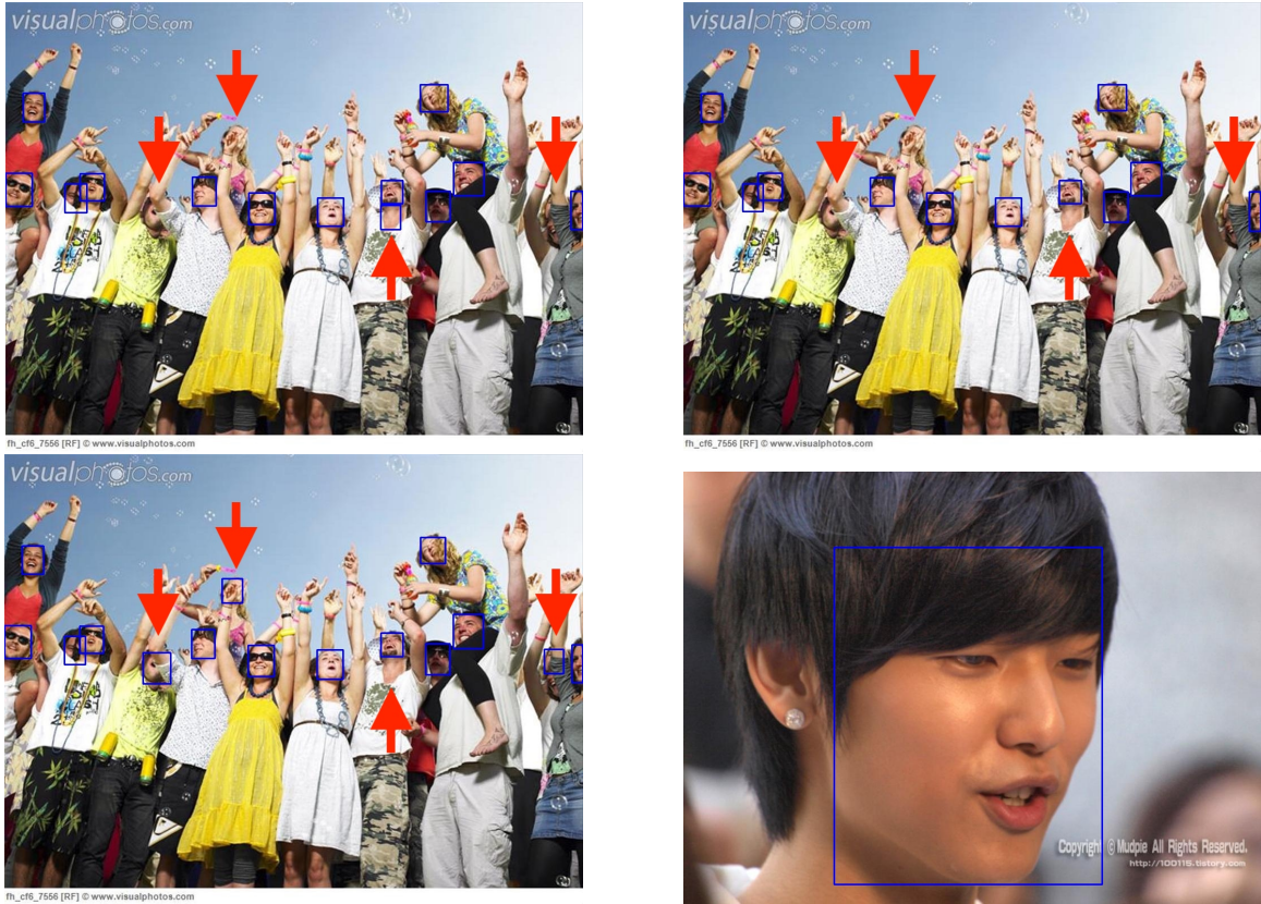
Figure 5.12. Qualitative example. Left-upper: baseline. Right-upper: +DH. Left-lower: +DH+HIM. The first three subfigures are the results on the same image, and the differences are highlighted by red arrows. Right-lower: Large face detected by our final model. Detected boxes with scores greater than 0.5 are plotted.
